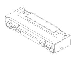
The 11501 Series is a 0.5mm pitch NON-ZIF RA type FFC connector. Compatible with FFC with shield that enables high-speed transmission of digital signals. A shield is attached and EMC measures are also taken. The optimized contact structure supports up to 20Gbps transmission range by selecting FFC. (Representative reference value defined by the company) Impedance matching: Differential  $100\Omega$
