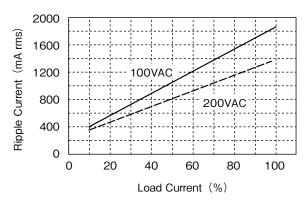
Fig. 1-2-(1) Ripple current value for PFE500F Series (A value per one of Fig. 1-1-(1) connection)
