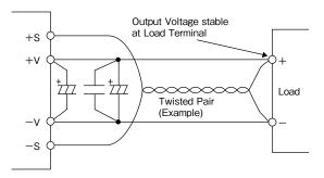
Fig. 9-1 Remote Sensing is used
