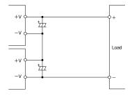
Fig. 9-1 Series Operation for High Output Voltage Applications
