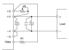
Fig. 2-1 External Resistor Connection Example
