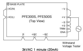
Fig.17-2 Input to Output Withstand Voltage Test Method
