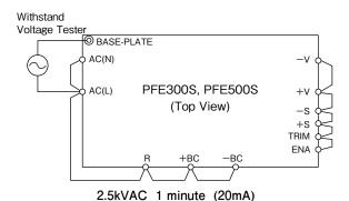
Fig. 17-1 Input to Baseplate Withstand Voltage Test Method
