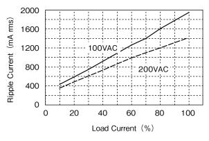
Fig. 1-2-(2) Ripple current value for PFE1000F Series (A value per one of Fig. 1-1-(2) connection)
