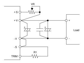
Fig. 2-1 External Resistor Connection Example
