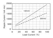
Fig. 1-2 Allowable ripple current value
