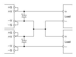
Fig. 10-2 ±Output Series Applications
