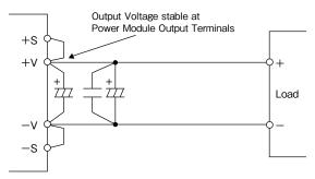
Fig. 9-2 Remote Sensing is not used (Local Sensing)
