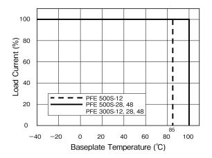
Fig. 12-2 Derating Curve
