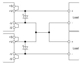
Fig. 11-2 +/-Output Series Applications
