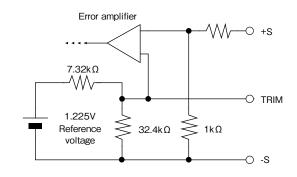
Fig.2-3 Internal TRIM Circuit (For the Reference)
