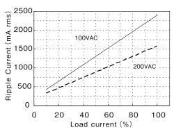
Fig. 1-2 Allowable ripple current value
