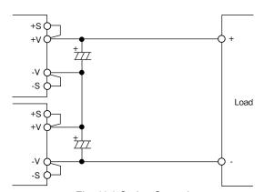
Fig. 11-1 Series Operation for High Output Voltage Applications
