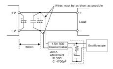
Fig. 2-1 Output Ripple Voltage (including Spike Noise)
