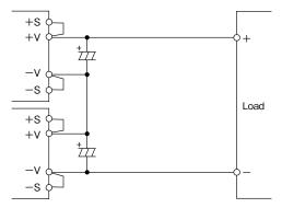
Fig. 10-1 Series Operation for High Output Voltage Applications
