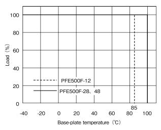
Fig. 16-2-(1) PFE500F Series Derating Curve
