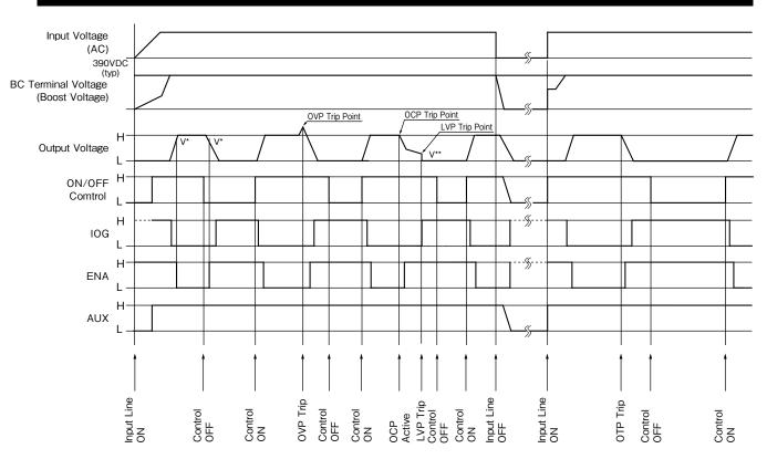
$V^{\star}$  voltage level: Refer to Application Notes "13.Power ON Signal" section.
