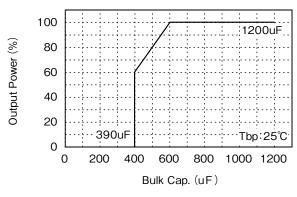
Fig. 1-3-(1) Output Power v.s. Boost Voltage Bulk Capacitance For PFE500F Series
