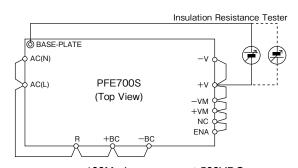
100M ohm or more at 500VDC Fig. 17-1 Insulation Resistance Test Method
