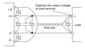
Fig. 9-1 Remote Sensing is used
