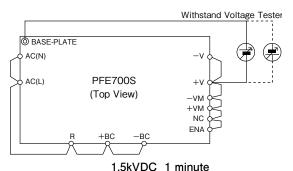
Fig.16-3 Output to Baseplate Withstand Voltage Test Method
