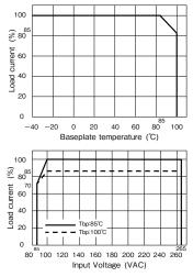
Fig. 11-2 Derating Curve
