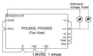
Fig.17-3 Output to Baseplate Withstand Voltage Test Method
