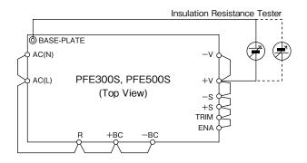
$100 M\Omega$  or more at 500 VDC Fig. 18-1 Insulation Resistance Test Method
