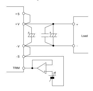
Fig. 2-2 Output Voltage Adjustment by applying external voltage
